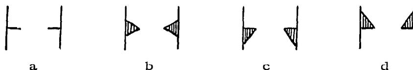
Fig. 1. Restricting devices. (a) Gradually diminishing openings spaced 25 cm apart; also tested with identical openings of 10 mm spaced 7 cm apart; (b) conical and (c) and (d) semiconical shapes; openings of 10 mm, tried under several spacing conditions.
